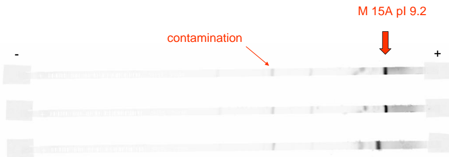
Figure 11. Fluorescein pI marker 15A focused on 3-10 NL 18 cm strips in the presence of 10, 100, 200 µg of E.Coli peptides (from the bottom top). The other bands in the image represent contaminations.
