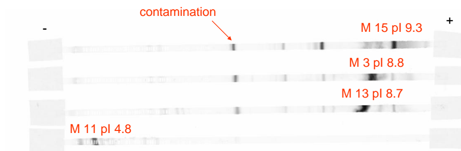
Figure 9. Fluorescein pI markers 11, 13, 3, 15 focused on 18cm 3-10 NL strips in the presence of BSA peptides. The other bands in the image represent contaminations.
