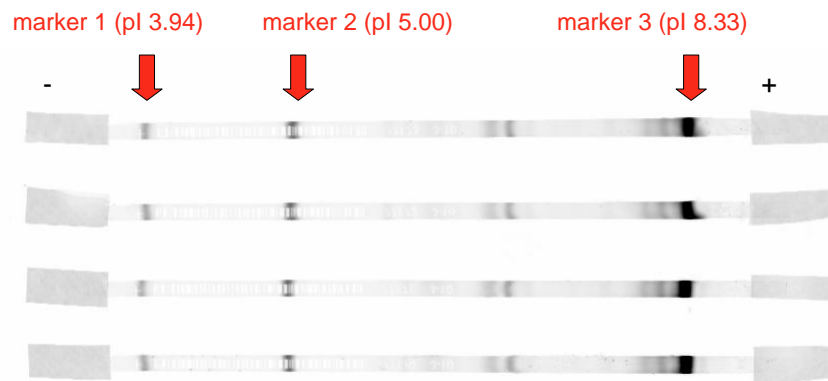
Figure 8. Fluorescein pI markers 1, 2, and 3 focused on 3-10 L 13 cm strips in the presence of S. aureus S 30 peptides H(-) first two from the top, and in the presence of S. aureus S 30 peptides H(+) first two from the bottom.
